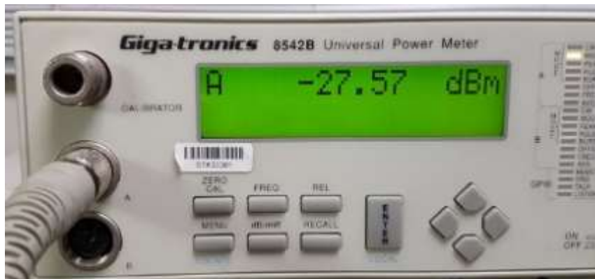
Figure 10: 3.84GHz output cold start (note that this is almost 10dB lower then what other guys have measured)
