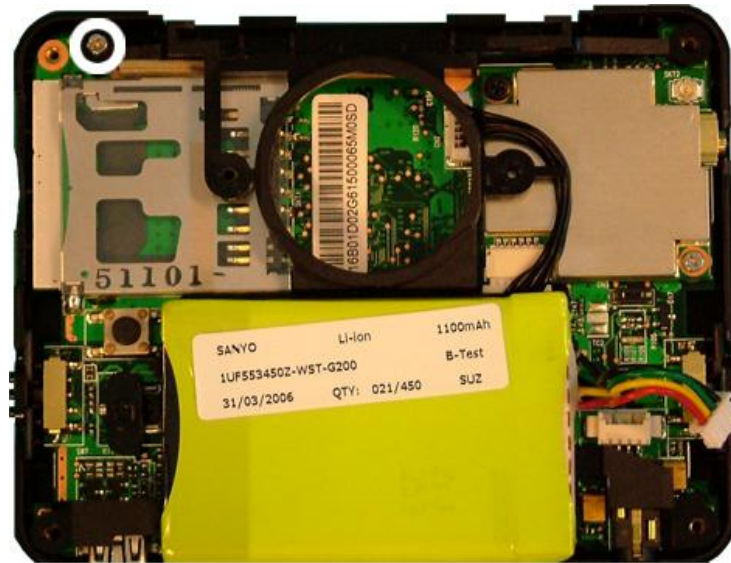
Fig. 5 The screw that keeps the antenna holder in place.
