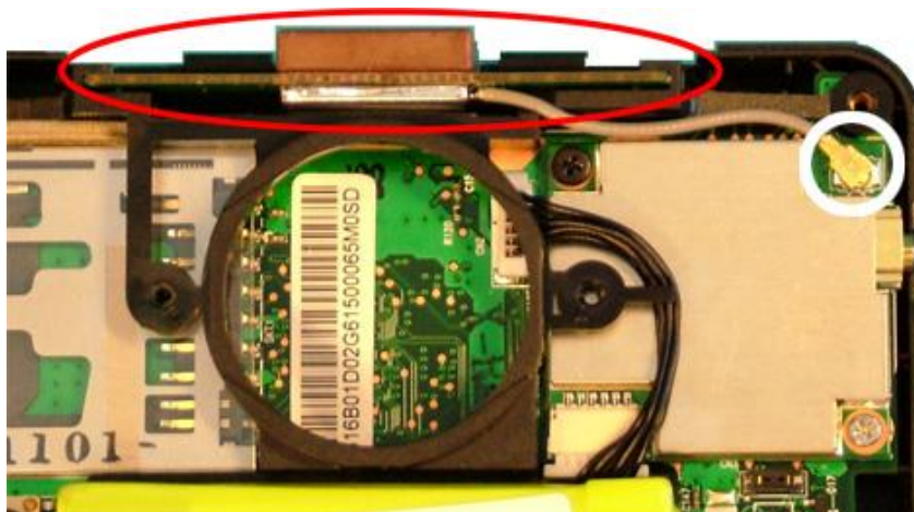
Fig. 4 The GPS antenna and cable connector.
