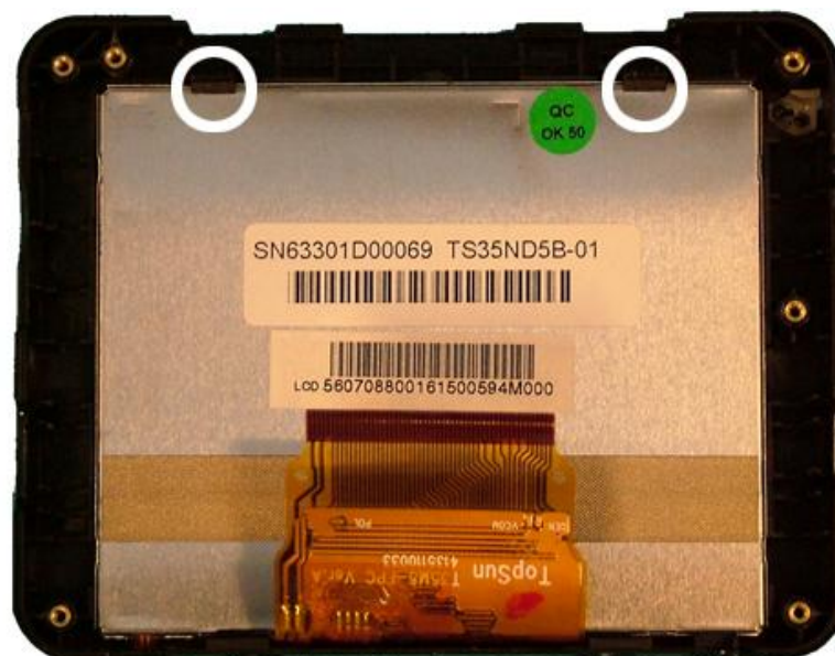
Fig. 8 LCD panel and front cover.
