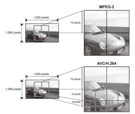
Compared to MPEG-2 compression, H.264 divides the image into smaller pixel blocks for higher picture quality
