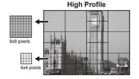
Main Profile: Fixed process is applied using 4 x 4-pixel blocks.
