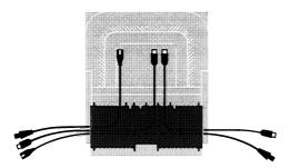
Arrange the connector cables in the cable cover as shown.
