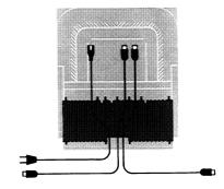
If you intend to place the loudspeakers further away from the centre unit, the connector cables should be run as shown here.
