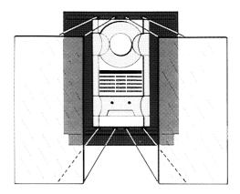
Note: Treat the glass doors with care! If they crack or chip or if they are damaged in any other way, they should be replaced immediately as they could otherwise cause bodily harm. You can order replacement doors through your Bang & Olufsen dealer.
