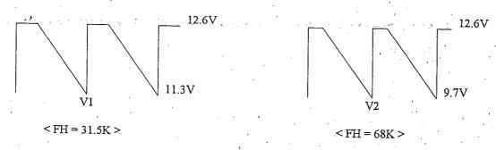
fH = 31.5K as V1 voltage goes lower, the Q501 Vc discharges slower in less oscillation range fH = 68K as V2 voltage goes higher, the Q501 Vc discharges faster in more oscillation range
