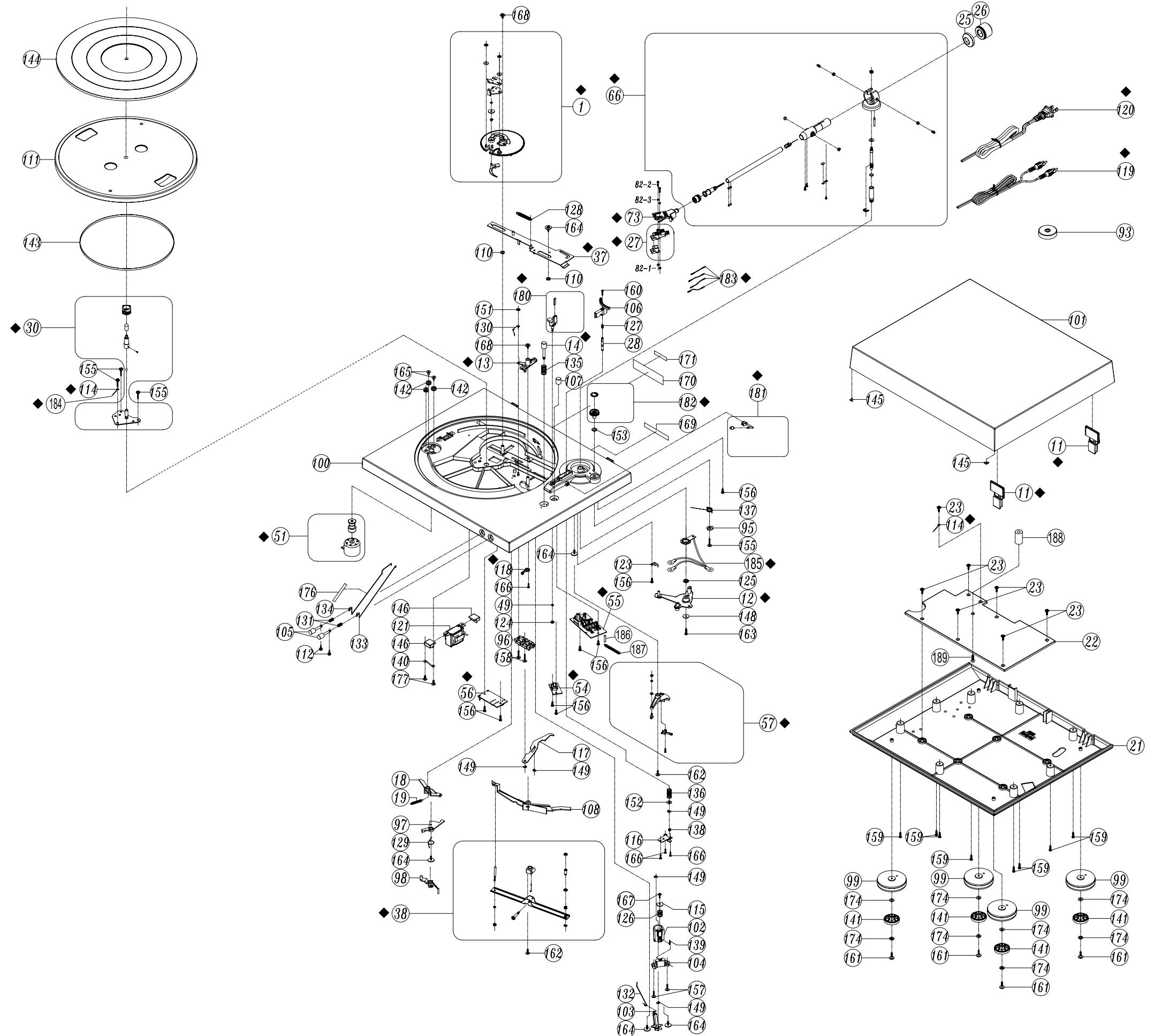
You have to remove the parts that marked "WEEE mark ♦" when the recycling processing.
