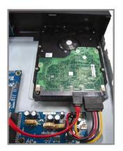
Step4: Align the screw hole on the each bracket with the screw hole on the each side of the HDD as shown below, and fix the HDD to the bracket with a HDD screw supplied.
