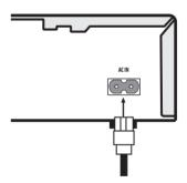
Plug the supplied AC power cable into the AC IN inlet and the other end into a standard household power outlet.
