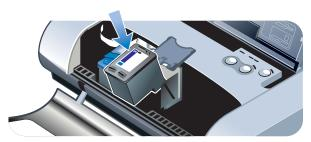
5 Close the print cartridge latch. If the cartridge is inserted correctly, closing the latch gently pushes the cartridge into its socket. Press the latch to make sure it is seated flat on the cartridge.
