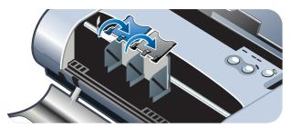
4 Insert each print cartridge into the correct socket (HP No. 57 in the left socket; HP No. 56 or 58 in the right socket). Make sure you insert the print cartridges at a slightly tilted back angle.
