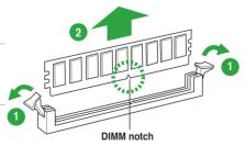
2. Remove the DIMM from the socket.
