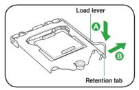
Lift the load lever in the direction of the arrow until the load plate is completely lifted.
