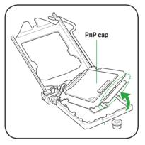
Position the CPU over the socket, ensuring that the gold triangle is on the bottom-left corner of the socket, and then fit the socket alignment keys into the CPU notches.
