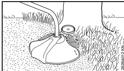
A depth wheel can be quickly fitted to the trimmer (see "Mounting Depth Wheel").
