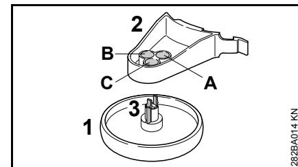
The depth wheel (1) can be locked in three different positions (A, B or C) on the support (2). This allows the reach of the mowing line to be varied.
