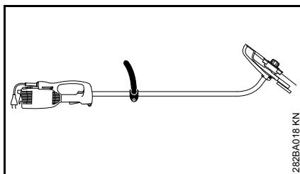
The trimmer can now be turned through 180° and used as a power edger (see "Applications").
