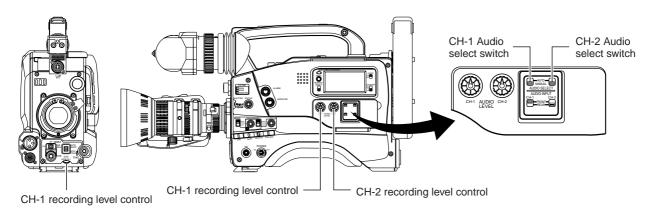
For each audio channel, use the AUDIO SELECT switches to select whether the recording level adjustment should be set to AUTO mode or MANUAL mode.
