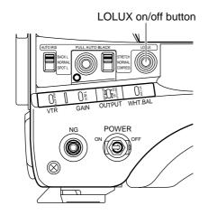
The LOLUX button is used when the illumination is still insufficient after compensating with the GAIN switch.
