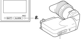
**8.** Press the VTR trigger button on the GY-DV500 or lens to start recording.
