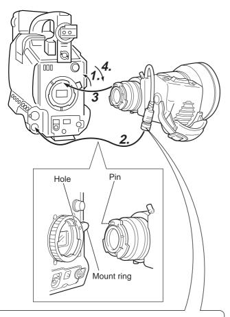
When unplugging the cable connector, first remove the lens itself. Then grasp this portion and pull straight out.
