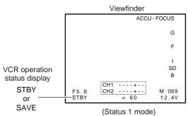
When a recordable videocassette is loaded, the GY-DV500 enters the record-pause mode. However, the record-pause operation condition differs depending on the setting of the VTR switch.
