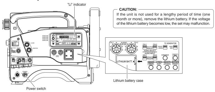
When the lithium battery is not in place or the battery is exhausted and requires a replacement, the "Li" indicator in the LCD display will light up.
