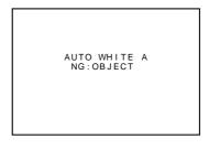
In the case of troubles occurring during operation of the GY-DV500, it performs a self-test to identify the cause and displays the result in the form of an error code. The error code consists of the "main code" which indicates its contents and the "sub-code" which indicates the details. Depending on the status of the GY-DV500 at this time, indications may also appear on the LCD display, the WARNING indicator may activate and the alarm tone may be generated.
