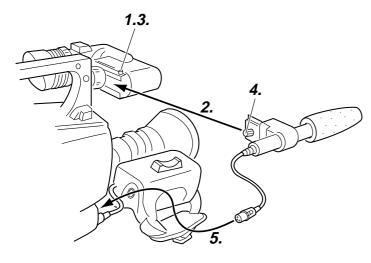
Connecting the provided microphone to the viewfinder. The provided microphone is a phantom microphone.
