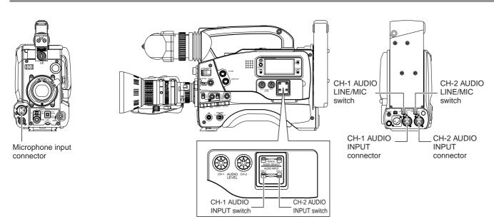
The GY-DV500 is provided with the microphone connector on the front section and the two AUDIO INPUT connectors at the rear section for audio input.
