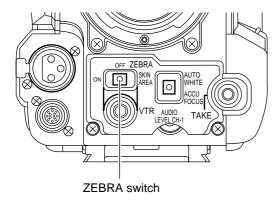
By setting the ZEBRA switch to  ${\bf ON}$ , oblique stripes (zebra pattern) can be displayed in the sections with a luminance level of 70% to 80% or sections with levels over 100% in the viewfinder.
