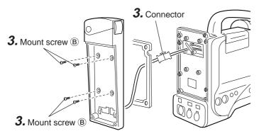
**3.** To remove the battery case, remove the four screws (B) fixing the battery case and the connector connecting the battery case to this unit.
