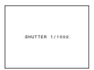
When the SHUTTER dial is pressed, a shutter speed is displayed (for approx. 5 sec.). In addition, whenever the shutter speed is altered by using the SHUTTER dial, the shutter speed is displayed. While this display is shown, other displays disappear.
