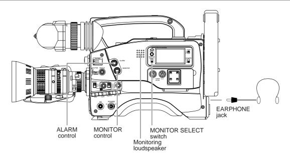
The audio input during recording, in record-pause or stop mode can be monitored through the monitoring loudspeaker or earphone.
