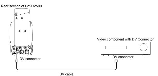
When connecting the GY-DV500 to a non-linear editing controller or other component with DV connector, be sure to observe the following procedure.
