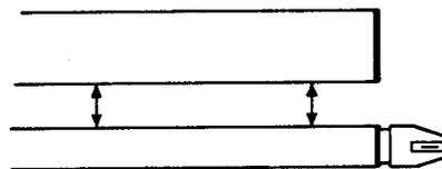
Adjust with the screw C until the pickup arm is parallel with the indicator arm.
