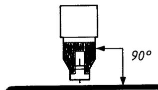
When exchanging pickup arms, the pickup parallelism is factory adjusted.
