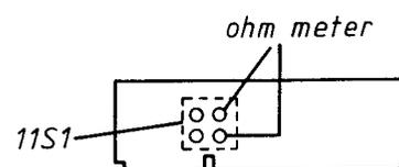
Connect an ohmmeter to the muting switch as shown, or pin 2 and 3 on the DIN cable.
