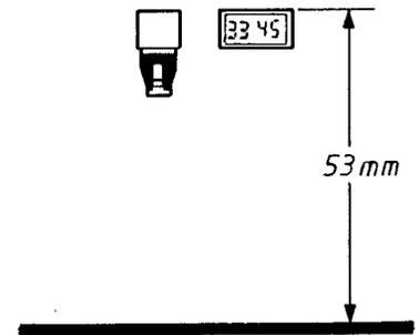
Adjust with the screw A until the distance is 53 mm from the topside of the indicator arm (at the outer end of the arm) to the swing chassis.
