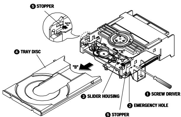
Fig. 3-9 Removing the Tray Disc
