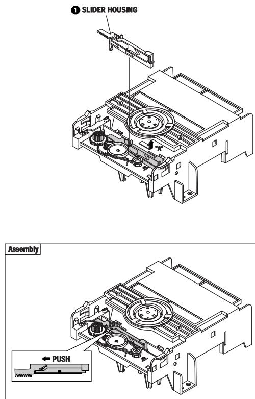
Fig. 3-10 Removing Slider Housing
