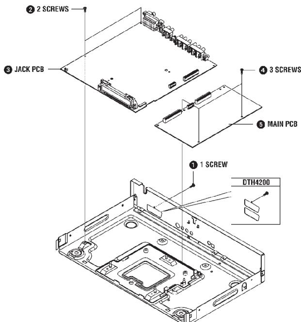
Fig. 3-5 Removing Main PCB and Jack PCB
