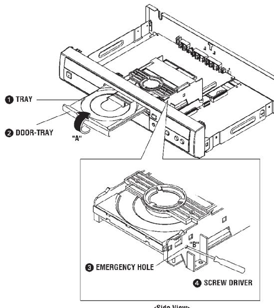
Fig. 3-2 Removing Door-Tray
