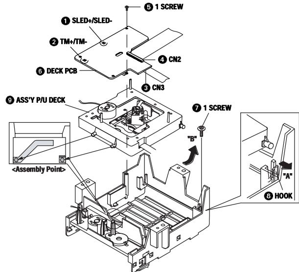
Fig. 3-8 Removing PCB Deck Assembly, P/U Deck
