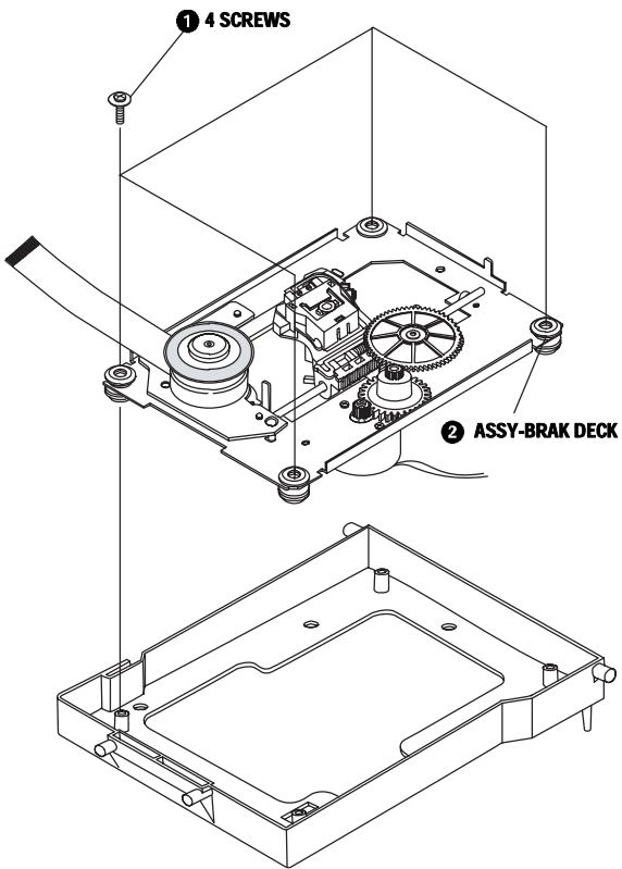
Fig. 3-5 Removing Sub Chassis
