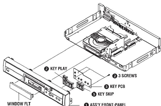
Fig. 3-3 Removing Assembly Front-Panel and Key PCB
