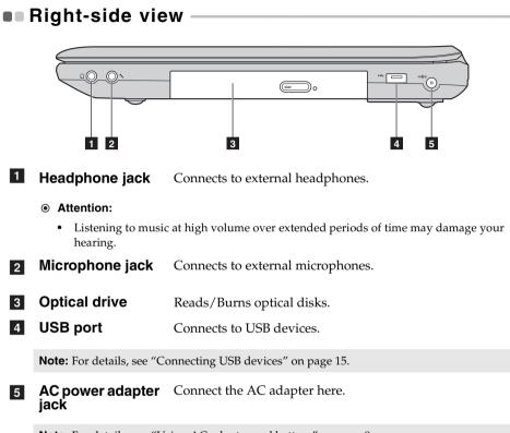
Note: For details, see "Using AC adapter and battery" on page 9.
