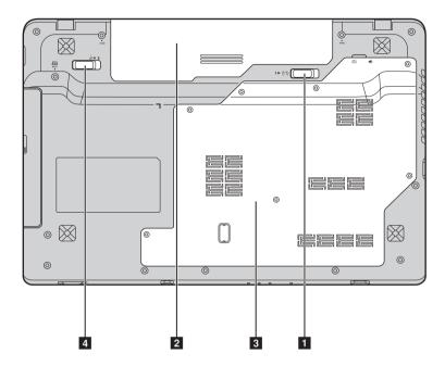
**Battery latch -**<br/>manualThe manual battery latch is used to keep the battery pack<br/>secured in place.
