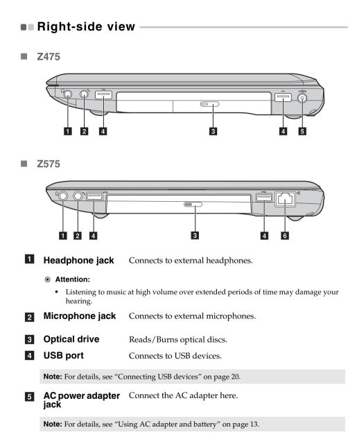
**6 RJ-45 port** This port connects the computer to an Ethernet network.
