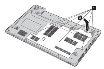
S Remove the frame fixing screws 3.
