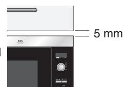
6. Fix the oven in position with the screws provided.
