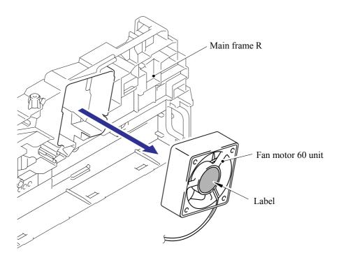
**CAUTION**: When re-assembling the fan motor 60 unit, make sure to turn the side with a label outwards.
