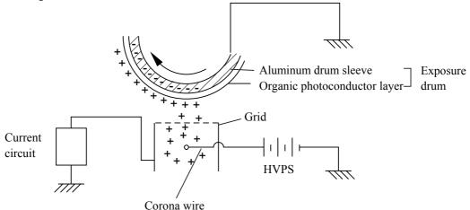
The primary charge uses a corona wire, but since the drum is positively charged, only less than 1/10 of the usual quantity of ozone is generated compared with the negatively charged drum. The level of ozone expelled from the printer is therefore not harmful to the human body. Applicable safety standards have been complied with.
