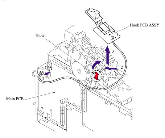
(3) Remove the actuator hook from the hook PCB ASSY.
