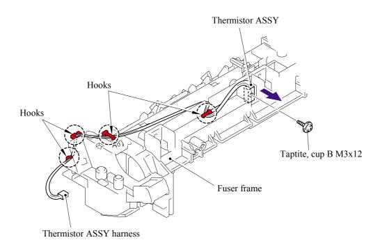
**NOTE**: When re-assembling the thermistor ASSY to the fuser frame, ensure the direction of the thermistor ASSY is correct referring to the figure below;
