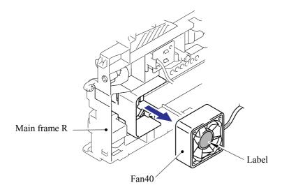
**CAUTION**: When re-assembling the fan motor 60 unit, make sure to turn the side with a label outwards.
