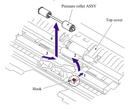
(15)Remove the two pressure rollers from the pressure roller shaft.
