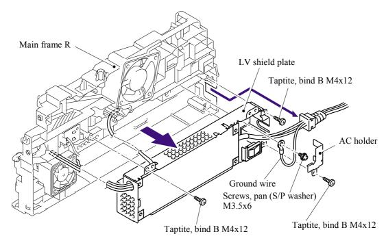
**NOTE**: Re-assemble the ground wire so that the section attached to the terminal is downwards.
