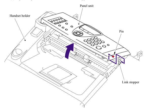
(2) Release the four hooks to remove the handset holder.
