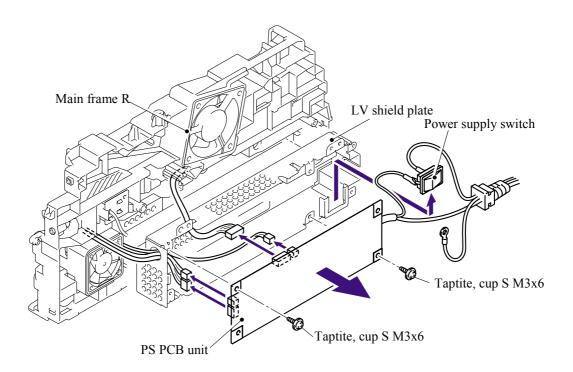
**NOTE**: When disconnecting the connectors, disconnect the regist sensor PCB connector and toner LED PCB unit ASSY connector first, lift up the PS PCB unit from the LV shield plate, and disconnect the main PCB connector.
