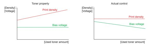
To always obtain a print result of a constant density, the printer counts the number of print pages immediately after the toner cartridge is replaced and changes the bias voltage according to the accumulated number of prints with the toner cartridge.
