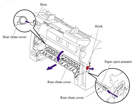
(2) Remove the paper eject actuator and the eject actuator spring.
