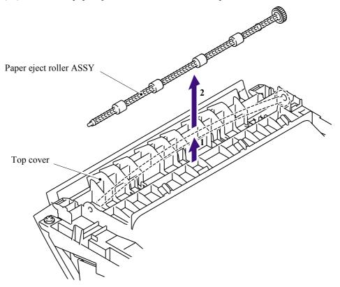
**NOTE**: When removing the paper eject roller ASSY, the spacer may come off easily. Be sure not to lose it.
