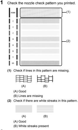
2 The confirmation screens for white streaks and missing lines are displayed alternately. Select the pattern that is closer to the nozzle check pattern that you printed.
