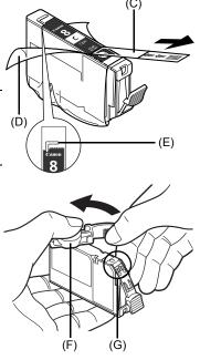
(F) Carefully hold the protective cap when removing it to prevent the ink from staining your fingers.
