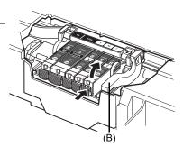
(B) Do NOT touch the Print Head Lock Lever; remove only the ink tank.
