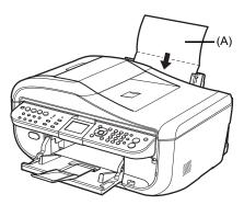
(A) Load the paper after unfolding it.
