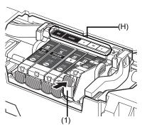
(H) Make sure the position of the tank matches the label.
