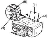
Do not load higher than the Load Limit Mark (B).
