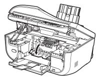
(1) Push the tab and remove the ink tank.
