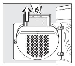
Open the door and pull the fluff filter out of the door as illustrated.
