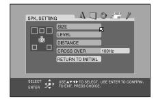
There are four items on the Speaker Setup Menu to configure the RSDX-02 for proper operation with your system. These adjustments can also be made from the front panel and/or remote control as described in the Sound Settings section of the manual.
