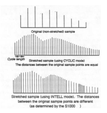
Select the sample to be stretched on the top line of the page, and then move down a line to select the part of the sample that you want stretched ("stretch zone" and "to").
