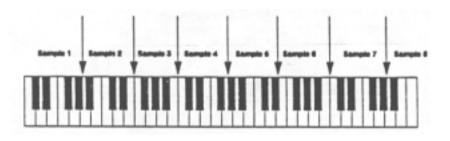
In this multi-sample program, there is no keyboard crossfading, so there may be audible jumps' between samples.
