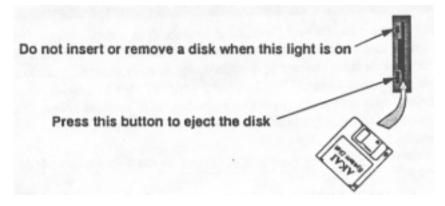
Insert the disk with the metal shutter first, and the label to the right
