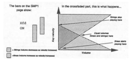
The neat parameter is "xfd" (crossfade) which may be either ON or OFF. If ON, any note which has a velocity which falls within two velocity zones will play both samples, the relative volume being adjusted accordingly.
