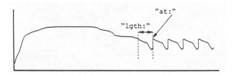
This is a poor choice of loop points. The sudden rise from the end of the loop to the beginning will cause audible "glitches"
