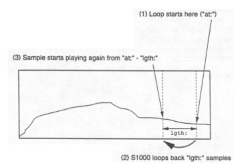
**Xfd:** This field determines the number of samples which will be cross-faded when the  $\underline{x}$ -<u>FD</u> button is pressed (see below).
