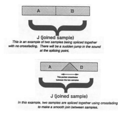
You can adjust the relative volumes of A and B by  $\pm 25$ dB, using the "scale" parameters. However, if you put these too high, you may get a distorted sound, so use these with care.
