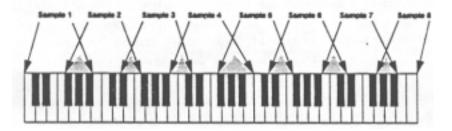
In this mufti-sample program, keyboard crossfading has been implemented. The gray triangles represent areas of crossfading, where two samples overlap, and a smoother transition is achieved at these points.
