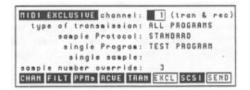
The first parameter, "channel", does not refer to a MIDI channel, but a "logical channel" used in System Exclusive protocol. Both samplers must be set to the same channel for transfer to take place.
