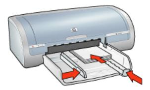
Large photographs: Place the photo paper in the In tray with the printable side down.
