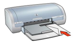
2. Push the envelope into the printer until it stops.
