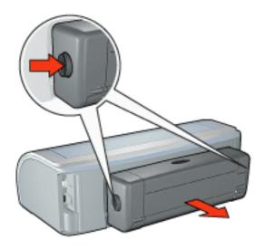
2. Remove any paper in the back of the printer.
