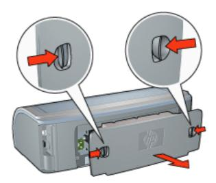
2. Remove the paper jam from the back of the printer, then replace the Rear Access Door.
