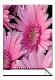
If the border appears above the tear-of tab, then <u>calibrate the printer</u>.
