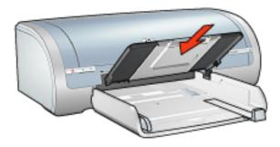
To prevent paper from falling out of the Out tray, pull out the Out tray extension.
