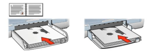
Tablet binding with portrait orientation: Reload the paper as shown below:
