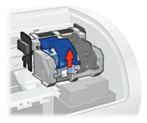
5. Slide the print cartridge out of the print cartridge cradle.
