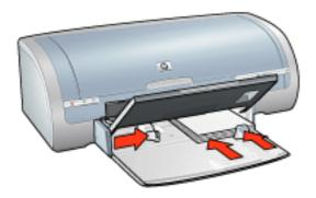
Large photographs: Place the photo paper in the In tray with the printable side down.
