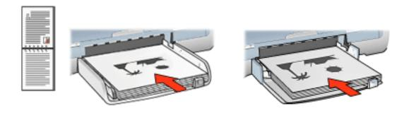
o Tablet binding with landscape orientation: Reload the paper as shown below:
