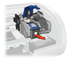
6. Remove the replacement print cartridge from its packaging and carefully
