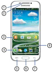
Light (RGB) and Proximity Sensors: Light sensor lets you use the ambient light level to adjust the screen brightness/contrast. Proximity sensor darkens the screen when held close to your face during a call.
