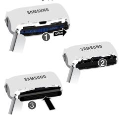
3. Rotate the battery cover downward and slide the battery cover release to the left (1) **CLOSE** position
