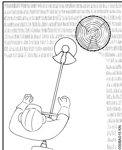
Mowing heads are to be used only on trimmer / brushcutters equipped with a line-limiting blade in the deflector in order to keep the line at the proper length (see "Main Parts" chapter in your instruction manual).
