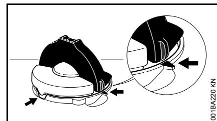
To do this with this STIHL cap, raise the grip on the top of the cap until it is upright at a 90° angle. Insert the cap in the fuel tank opening with the raised positioning
