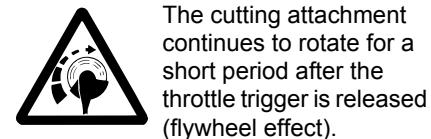
The cutting attachment continues to rotate for a short period after the throttle trigger is released (flywheel effect).
