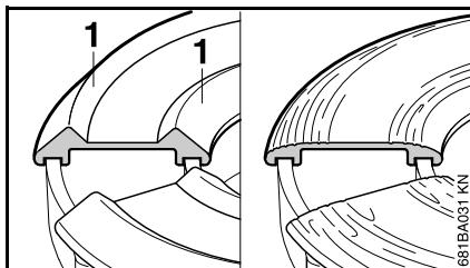
Do not continue using the mowing head if the raised moldings (1) on the base are missing or worn – see right illustration above. The mowing head
