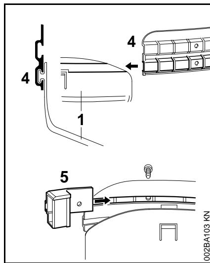
**⚠** These parts must be fitted to the deflector (1) when you use a mowing head.
