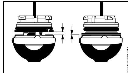
Left: Base of cap in closed position (with open space)
