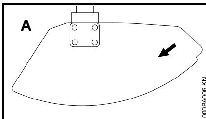
Arrows on the deflector (A) (as seen from the underside) show the correct direction of rotation of the cutting attachment. When viewed from above, however, the cutting attachment rotates counterclockwise.
