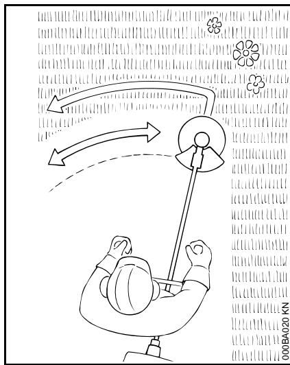
All kinds of grass and weeds can be easily cut with the grass cutting blade. The power tool is swept in an arc similar to a scythe.
