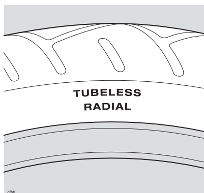
Typical Tyre Marking - Tubeless Tyre
