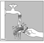
Clean the filter under a running tap, then refit it, screwing it fully in.
