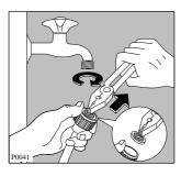
If you notice that the machine is taking longer to fill, check that the filter in the water inlet hose is not blocked.
