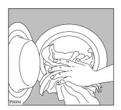
Open the door by pressing the — button and place the laundry in the drum, one item at a time, shaking them out as much as possible. Close the door.
