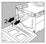
Remove the polystyrene blocks from the underside of the machine and release the two plastic bags by removing the adhesive strip. Unscrew and remove the feet. Carefully remove the right-hand bag (1) then the left-hand bag (2) by pulling them towards the centre of the machine.
