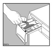
Pull out the dispenser drawer until it stops. Measure out the amount of detergent recommended by the manufacturer in a graduated cup and pour it into the main wash compartment []].
