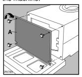
Fit the grid on the bottom of the machine and re-fit the feet.
