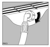
The other end of the inlet hose which connects to the machine can be turned in any direction. Simply loosen the fitting, rotate the hose and retighten the fitting, making sure there are no water leaks.
