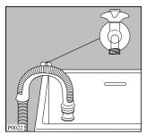
Hooked over the edge of a sink using the plastic hose guide supplied with the machine. In this case, make sure the end cannot come unhooked when the machine is emptying.
