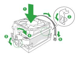
Align the other end of the retention bracket to the retention module base. A clicking sound denotes that the retention bracket is in place.
