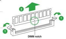
2. Remove the DIMM from the socket.
