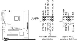
M4N68T-M Analog front panel connector
