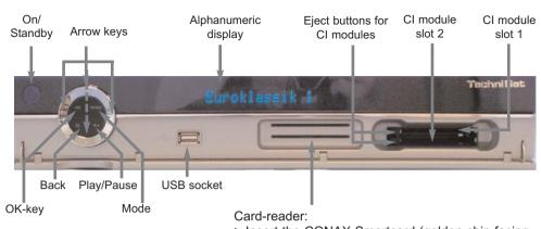
> Insert the CONAX-Smartcard (golden chip facing downwards and in the direction of insertion) until the point of contact in the card-reader.
