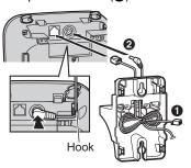
3 Insert the hooks on the wall mounting adaptor into holes (4) and (3) on the base unit.
