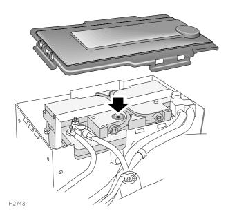
To access the battery, unclip and remove the battery cover as shown in illustration.
