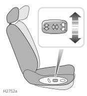
Push the front of the switch up or down to tilt the seat cushion to the desired position.
