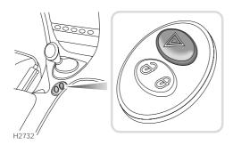
Press to operate. All the direction indicators and direction indicator warning lights will flash together. Use only in an emergency to warn other road users when your car is causing an obstruction or is in a hazardous situation. Remember to switch off before driving away.
