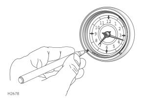
To adjust the time, use a ball point pen or similar probe to advance or put back the time, using the right or left hand buttons at the bottom of the clock bezel.
