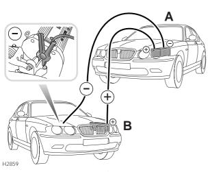
DO NOT connect a booster cable to the negative (-) terminal of the discharged battery!
