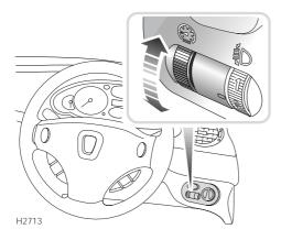
Rotate the control up to increase and down to decrease instrument illumination. The instrument dimmer also controls the illumination of switches, audio system, message centre, trip computer and the satellite navigation system (if fitted).
