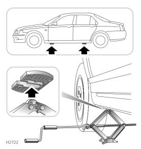
NEVER work beneath the car with the jack as the only means of support. The jack is designed for wheel changing only!
