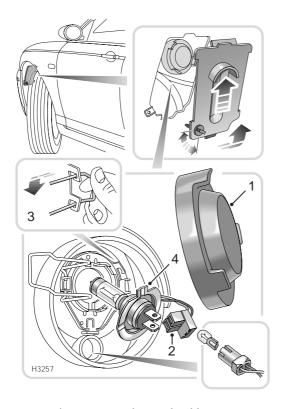
Using a screwdriver, rotate the turnbuckle a quarter turn to left or right to release the access panel. Push the panel up as far as it will go and then disengage the bottom of the panel to remove (see upper inset). It is then possible to reach the back of the combined headlight/sidelight unit.
