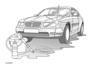
Some high pressure cleaning systems will penetrate door, window and sunroof seals, and damage lock mechanisms. DO NOT aim water jets directly at components that might be easily damaged.
