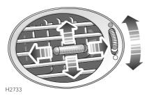
Rotate the thumbwheel down to close or up to open the vents. Direct the air flow by moving the control in the centre of the louvres up or down, or from side to side.
