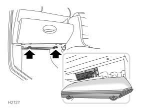
The passenger compartment fuse box is located behind the front passenger glove box.
