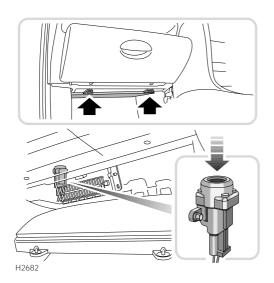
An inertia switch, operational only with the alarm disarmed, will unlock the doors in the event of an accident or sudden impact.
