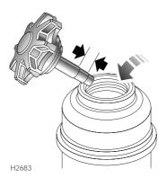
Fluid specification: Use any fluid to Dexron III specification. Fluids manufactured to this specification are suitable for use in temperatures between -20° C to +30° C (if climatic temperature falls outside these limits, seek advice from your dealer).
