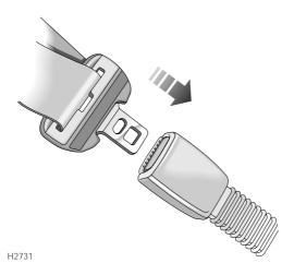
Pull the seat belt steadily over the shoulder and across the chest and, ensuring the webbing is not twisted, insert the metal tongue plate into the appropriate buckle – a 'click' indicates that the belt is securely locked.
