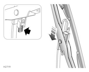
Lift the wiper arm away from the windscreen and set the blade at 90° to the arm as shown. Disconnect the blade by pushing in the locking tab (arrowed in inset), setting the blade at 45° to the arm and sliding the blade down the arm.
