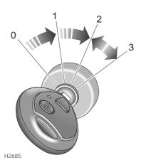
Once the steering lock is engaged, it is impossible to steer the car. DO NOT remove the key or turn the starter switch off while the car is in motion.
