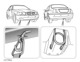
If your car is to be transported on the back of a trailer or transporter, use the recommended lashing points at the front and rear of the car only. DO NOT secure lashing hooks, 'T' bars or trailer fixings to any other part of the car.
