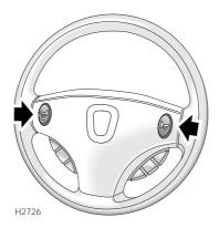
To operate, press either of the horn switches set into the steering wheel pad.
