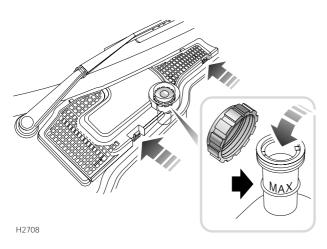
Remove the detachable mesh panel on the driver's side of the car to access the brake fluid reservoir. The fluid level can be seen through the reservoir neck and should be maintained as close to the 'MAX' mark as possible. DO NOT allow the level to drop below the 'MIN' mark.
