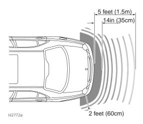
The parking aid is not infallible. It is for guidance only! The sensors may not be able to detect certain types of obstruction, eg. narrow posts or small objects no more than a few inches wide, small objects close to the ground, objects above the level of the boot and some objects with dark non-reflective surfaces.
