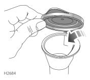
DO NOT use an anti-freeze or vinegar/water solution in the washer reservoir - anti-freeze will damage painted surfaces, while vinegar can damage the windscreen washer pump.
