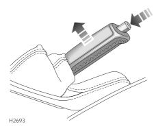
The handbrake operates on the rear wheels only. To apply the handbrake, pull the lever up. Always apply the handbrake FULLY whenever you park the car.
