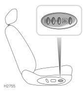
Your car can memorise three different driver seating positions. To store the positions in the system memory, the starter switch must be turned to the first or second position.
