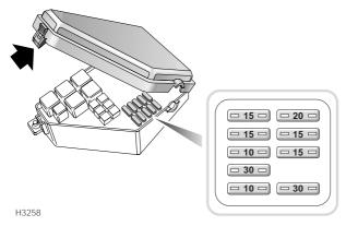
The fuse box is located on the left hand side of the engine compartment. Press the catch (arrowed in illustration) to release the hinged cover.
