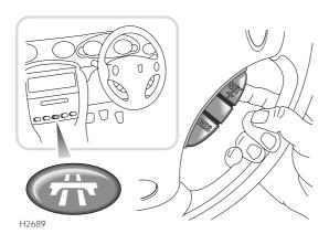
Cruise control enables the driver to maintain a constant road speed without using the accelerator pedal. This is particularly useful for motorway cruising, or for any journey where a constant speed can be maintained for a lengthy period.
