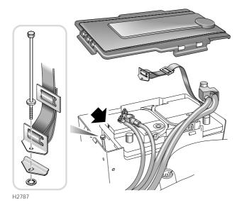
Disconnect the negative ('-') cable first and then the positive ('+') cable (when reconnecting, connect the positive cable first and then the negative cable).
