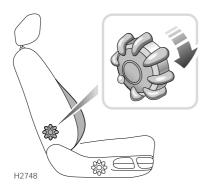
Rotate the handwheel to increase or decrease support to the lumbar region of the back.
