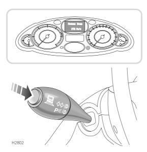
The trip computer utilises the message centre on the highline instrument pack only and provides valuable information to assist the driver to calculate fuel stops, journey times and distances.
