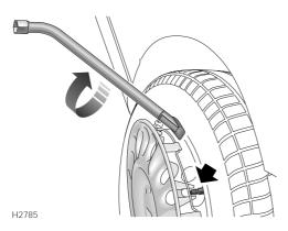
Slide the flat, wedge, end of the wheel wrench behind the edge of the wheel trim (see illustration). Then, working carefully around the wheel, apply a twisting action to the tool to prise the trim from the wheel.
