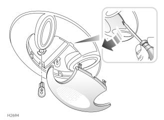
Insert a small flat-bladed screwdriver into the indent at the rear of the lens (see inset) and gently prise the lens from the light unit. Pull the bulbs from their mountings to remove.
