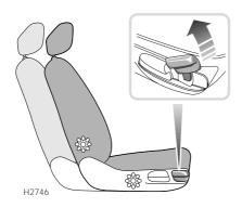
Your car is fitted with side impact airbags. Refer to the Airbag SRS section of this handbook before fitting seat covers, or carrying out any repair or retrimming operations to the seat or seat covers.
