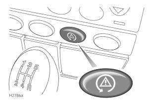
Operating tip: When driving with snow chains fitted, it is recommended that traction control be disabled.
