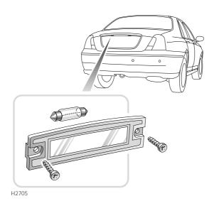
There are two number plate lights. To access each bulb, remove the two screws securing the lens and remove the lens.
