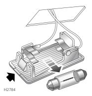
Insert a small flat-bladed screwdriver (preferably with a short handle, due to limited access) into the indent on the left hand side of the light unit, and carefully prise the unit from the glovebox panel. Remove the bulb from its clips.
