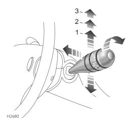
The wipers and washers will only operate when the starter switch is in the first or second position.
