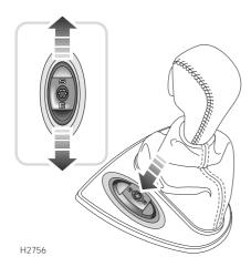
The automatic gearbox has three driver-selectable operating modes, Normal (economy), Sport and Snow. When the starter switch is turned on, the transmission automatically selects the Normal (economy) mode.
